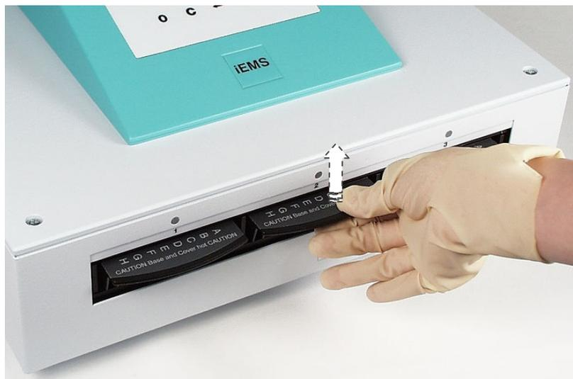
Fig. 6.5 Removing the microplate holder – lifting the handle
