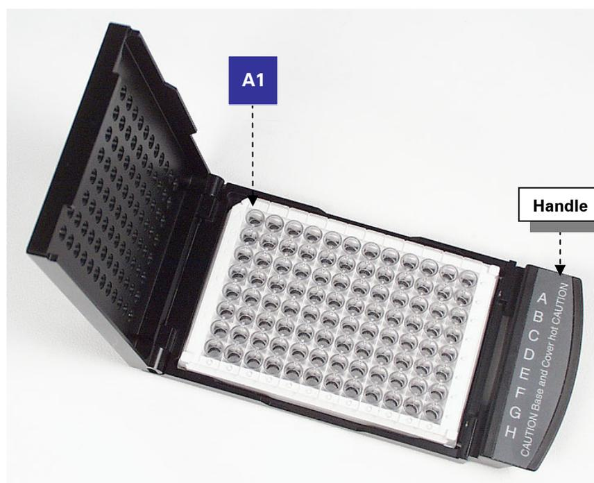
Fig. 6.2 Microplate in the thermal microplate holder
